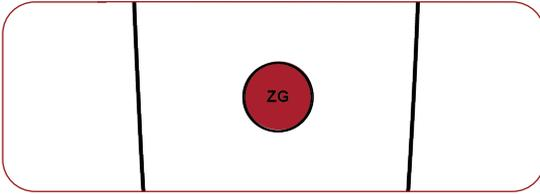
Press the ZG button (Zero Gravity) and release. This will fully recline the backrest and raises the footrest, placing your body in a neutral-posture position.
