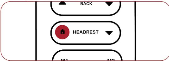
To return the seat to the starting upright position, simply press and hold the 🏠 HOME button until the chair is back to its original starting position.
